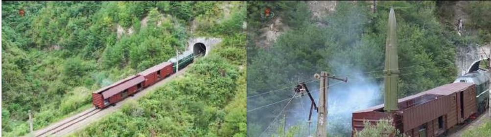
Figure 1. The DPRK rail-mobile launcher consisted of a locomotive, a supporting car and a missile launch car that accommodates two ballistic missiles.
