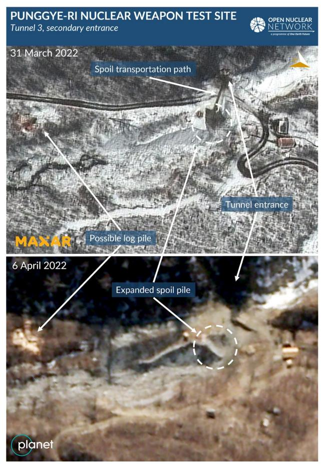
Figure 5. Comparison of the satellite images from 31 March and 6 April 2022 showing the spoil pile near the secondary entrance to Tunnel 3.
