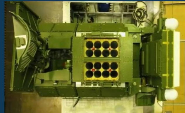
A Russian “Tor” system viewed from above. A total of 16 missiles are vertically stored between the search radar and fire control radar antennas. Image: en.topwar.ru
