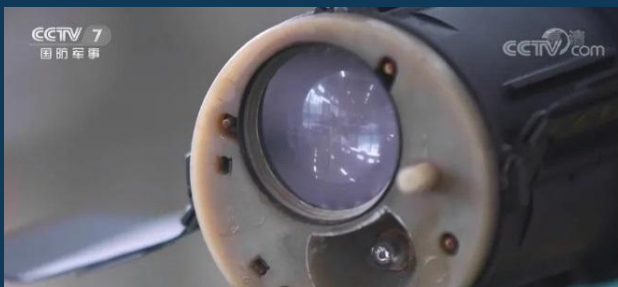
The rear end of a Chinese beam-riding ATGM. The sensor receives the laser, which is directed at the target, and keeps the missile inside the narrow beam. Thus, it "rides on" the beam and flies towards target. Image: China Central Television
