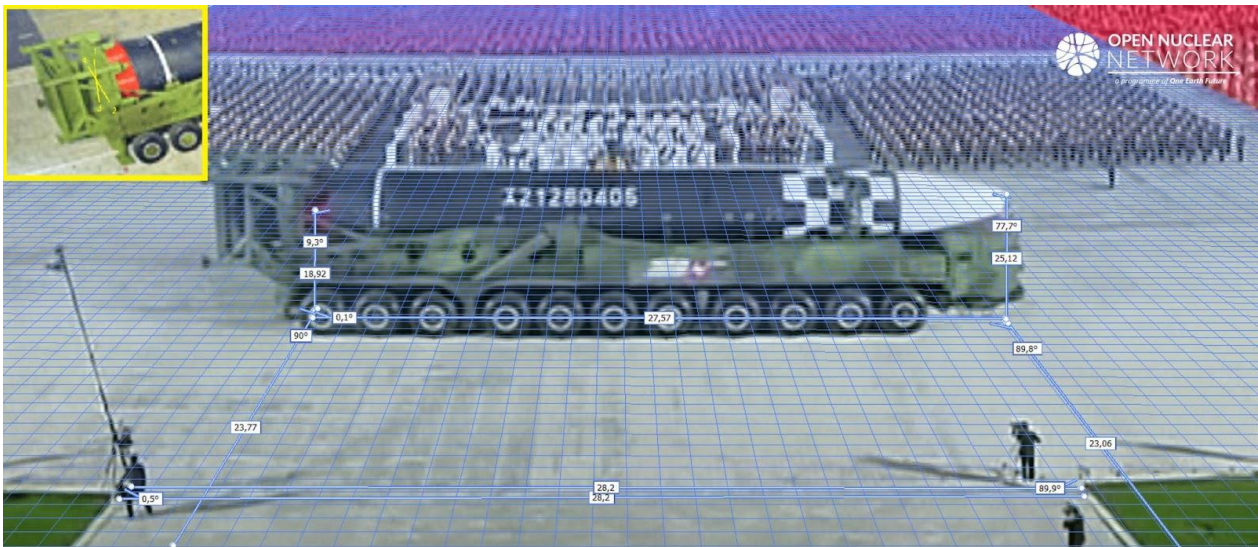
Figure 2. The missile's length and diameter can be estimated based on ground references that are also measurable in satellite imagery. Inset image: a red protective cover seems to show the contour of four engine nozzles.
