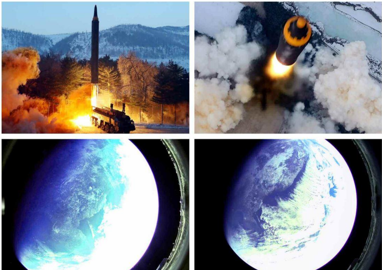
Figure 5. Hwasong-12 launched on 30 January 2022 (top). Camera view of the earth from the warhead (bottom). The images sent back to earth are proof that remote telemetry was working during the test. Images: Rodong Sinmun
