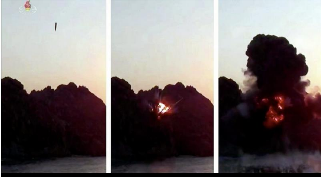
Figure 23. Angle of attack in the terminal phase of flight for the KN-24 116
