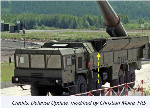
Figure 16. Relation between the diameter of the wheel of the MZTK 7930 launcher and the 9M720 SS-26E missile
