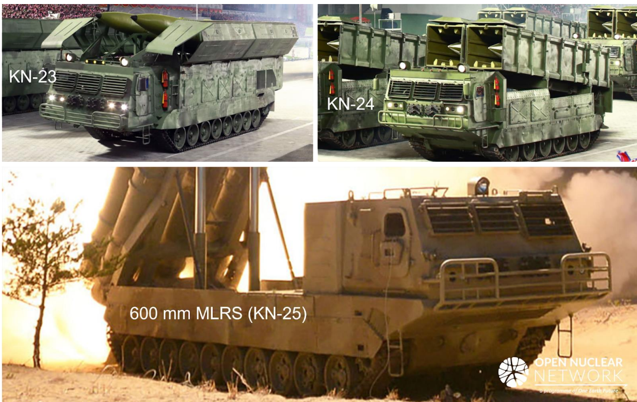
Figure 1. The tracked chassis of the 600 mm MLRS, with 10 road wheels on each side, is the largest of the new generation of short-range ballistic missile systems developed by the DPRK. In comparison, the tracked chassis of the KN-23 has eight road wheels on each side, while the tracked chassis of the KN-24 has six road wheels on each side.
