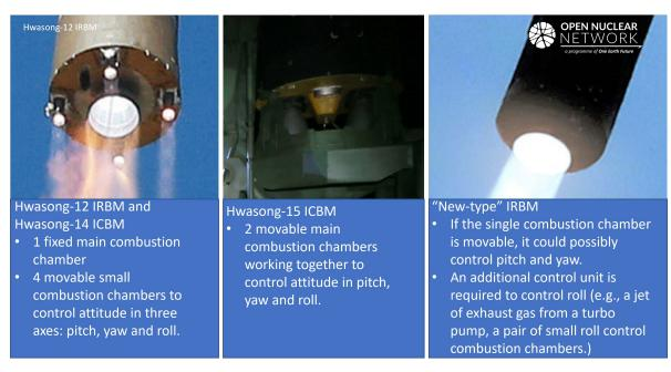
Figure 1. Comparison of the propulsion units between existing Hwasong strategic missiles and the "new-type" IRBM. Images: sogwang media corporation, KCNA, KCNA/Reuters[2]
