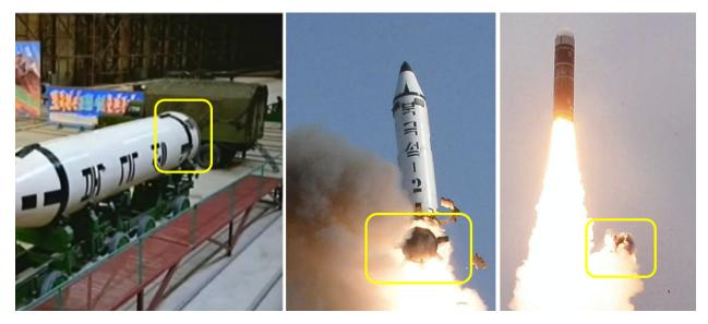
Figure 3. Gas generators, marked in yellow boxes, for the Pukguksong-1 SLBM (left), the Pukguksong-2 land-based ballistic missile (middle) and the Pukguksong-3 SLBM (right). Images: KCTV, KCNA
