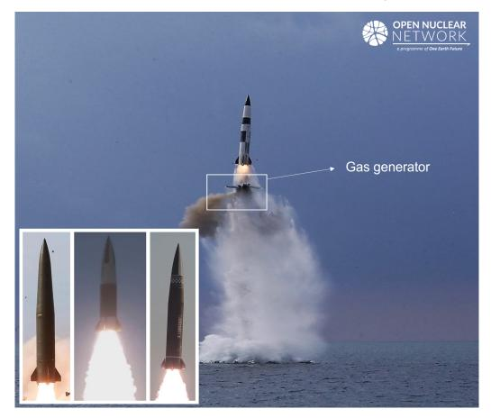
Figure 2. The gas generator was discarded after the new SLBM was ejected out of the water. Inset photos from left to right: KN-23, KN-24 and another SRBM tested by the DPRK on 25 March 2021. Image: KCNA, KCTV, annotated by ONN
