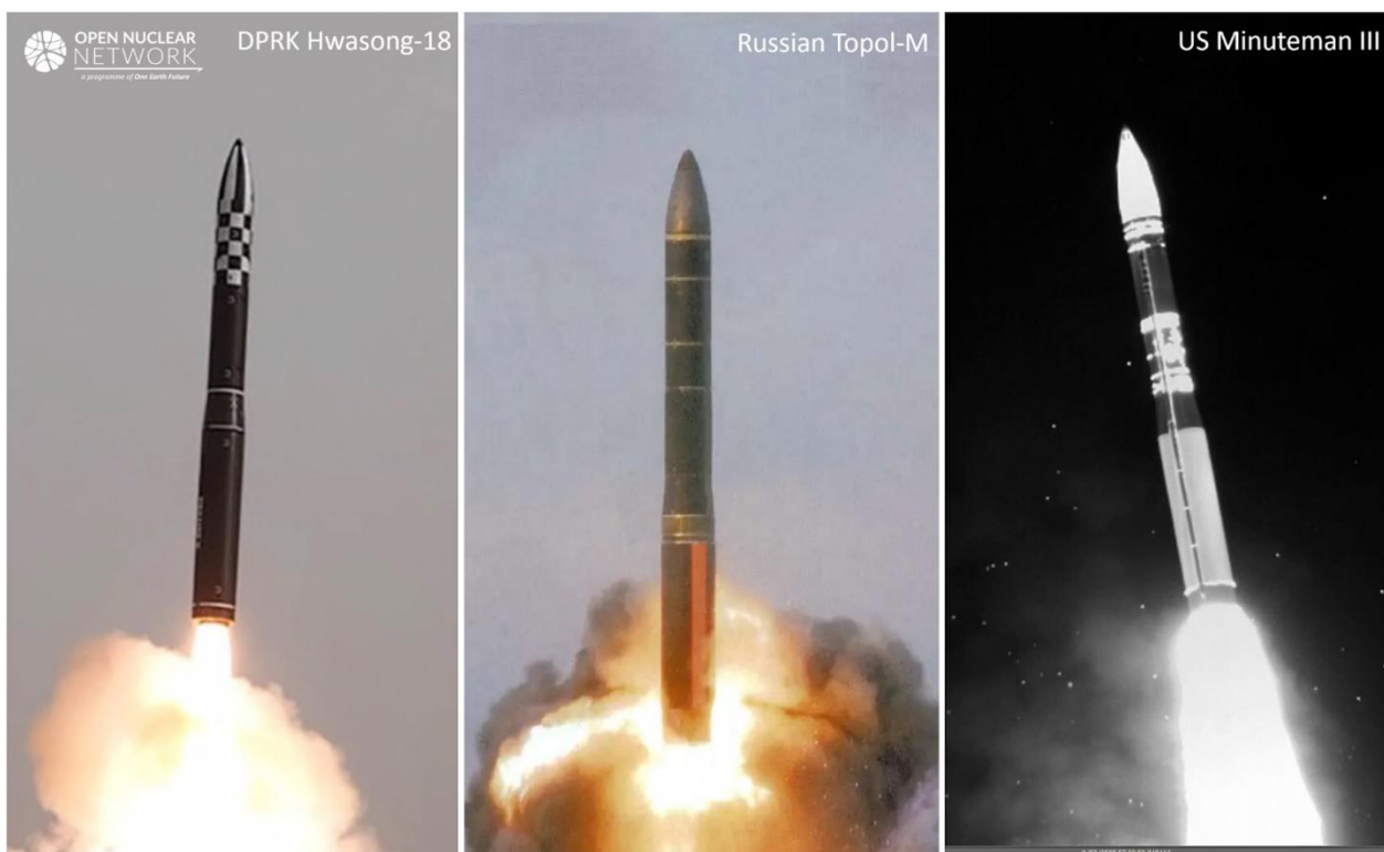
Figure 1. The Hwasong-18 has a typical solid-propellant ICBM layout similar to that of the Topol-M and the Minuteman III.
