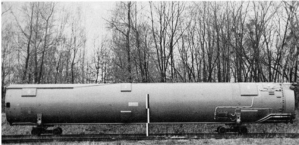
Figure 2. An ampoulized Soviet UR-100 ICBM in its transport-launch canister. Image: Russia's Arms Catalog 3
