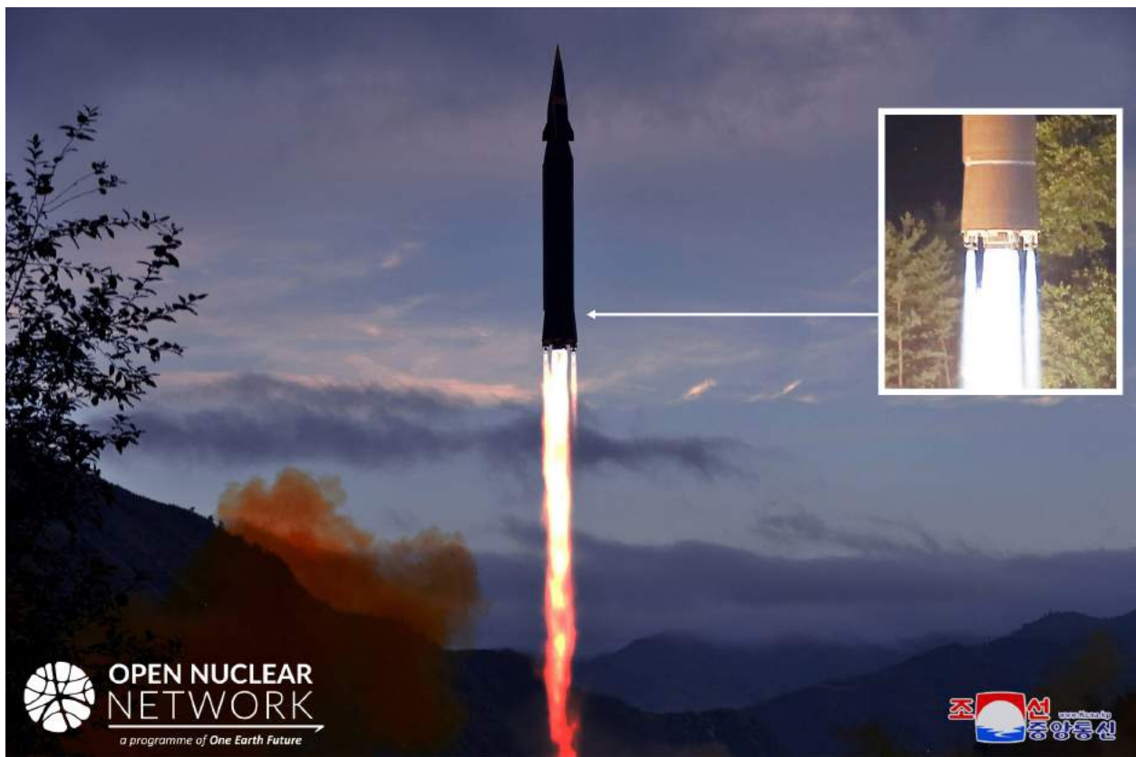
Figure 1. The engine powering the Hwasong-8 appears to have one main combustion chamber and four small combustion chambers to control flight attitude. Inset photo shows the engine section of the Hwasong-14 ICBM.
