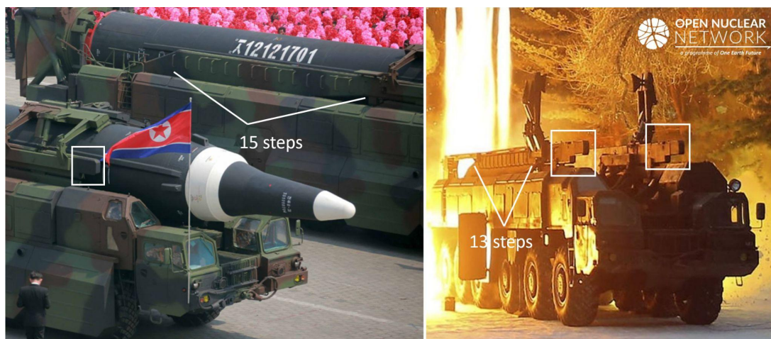
Figure 3. Hwasong-12 (left), hypersonic missile tested on 5 January 2022 (right). White boxes show the different lengths from the clips to the tips of the erection arms. Images: KCNA
