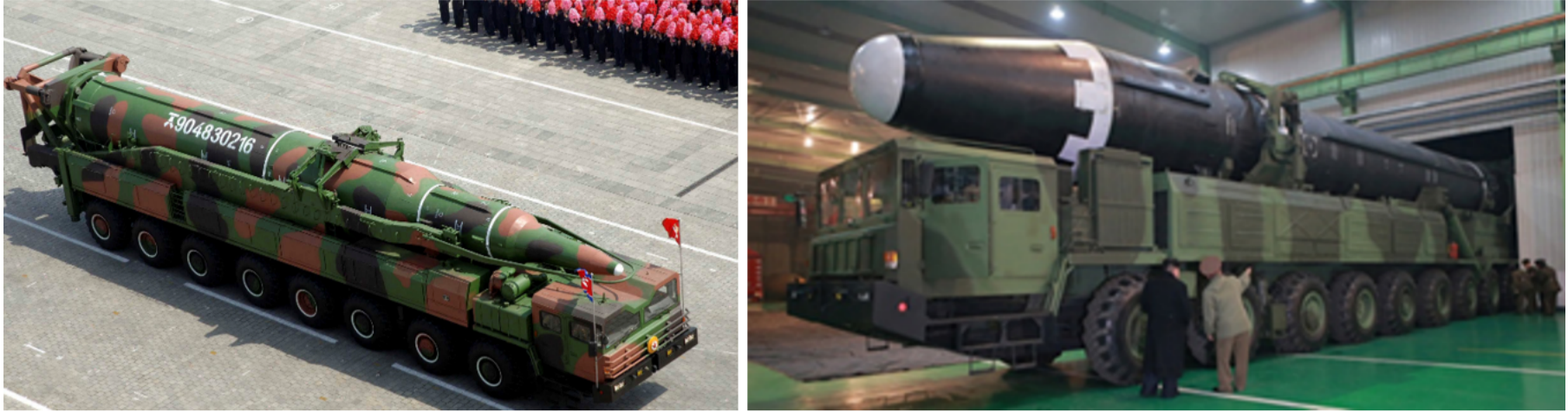
Left: Hwasong-13's first appearance during a military parade on a WS51200 adapted into a TEL. Right: Hwasong-15 on a WS51200 TEL further modified with a 9th axle. Sources: KCNA
