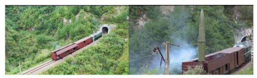
Figure 1. The DPRK rail-mobile launcher consisted of a locomotive, a supporting car and a missile launch car that accommodates two ballistic missiles.
