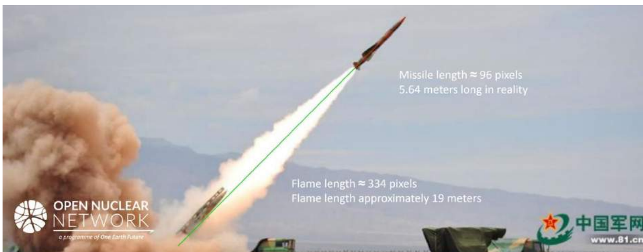
Figure 6. Measurement of flame length of an HQ-12 SAM using a photo taken at a favourable angle for measurement. 16 Image: 81.cn, annotated by ONN
