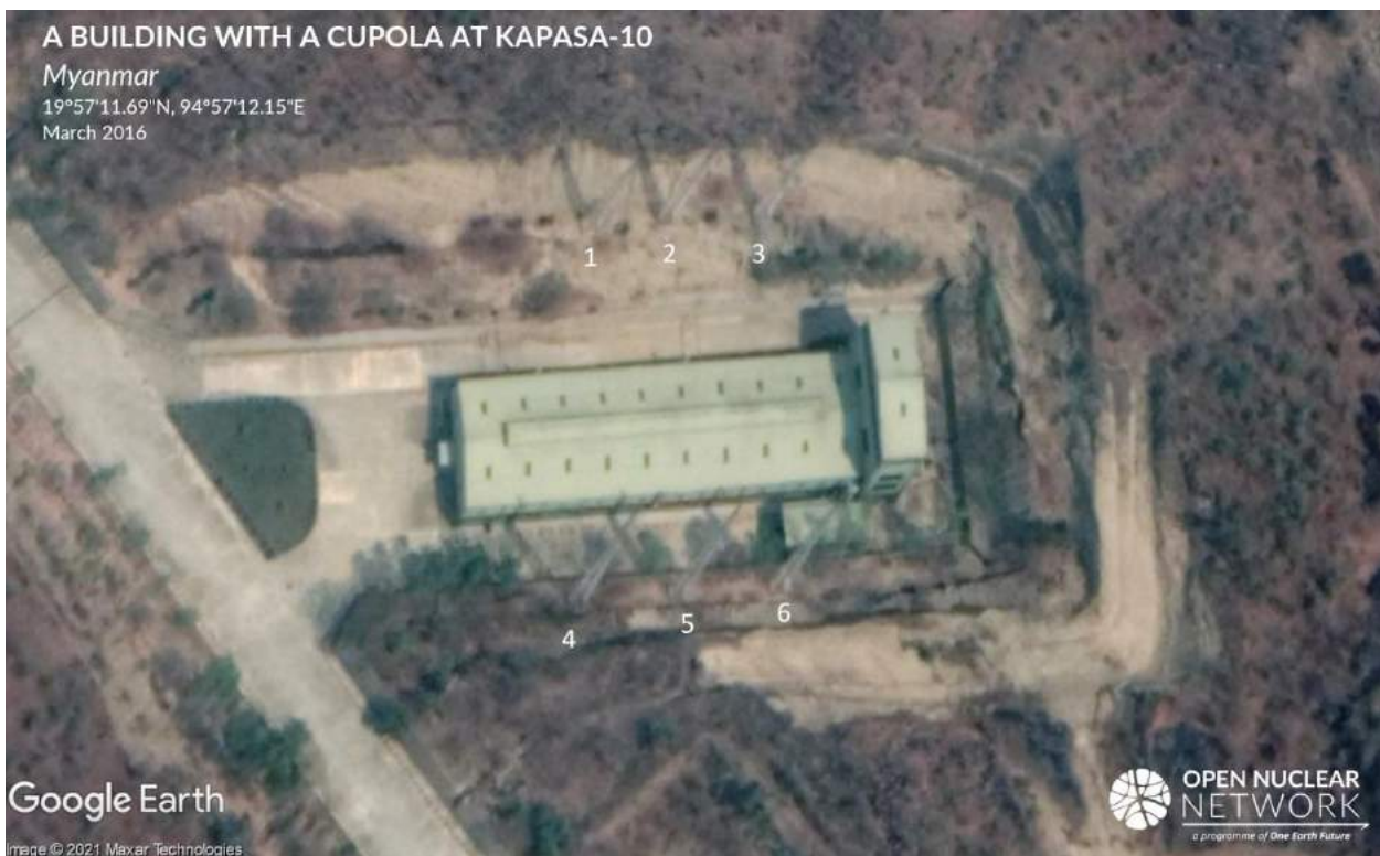
Figure 14. An elevated cupola at Kapasa-10 flanked by six lightning rods (marked in numbers). Image: Google Earth
